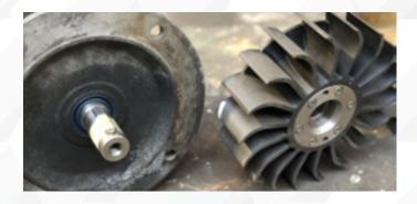
The 3D-printed turbine, boasting resistance to extreme mechanical stress, continues to operate flawlessly at high speeds (up to 1400 rpm) and continuous duty.
